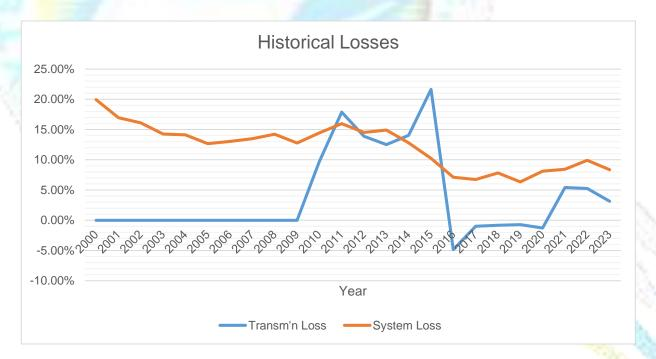
Historically, System Loss ranged from 19.94% to 6.34%. System Loss recorded at nearly 20% on year 2000. This is because of the distribution setup and long distribution lines that served by only few substations.
