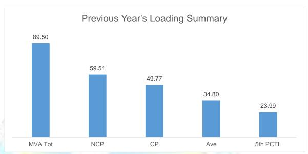
The Non-Coincident Peak Demand is 59.51 MW, which is around 66.49% of the total substation capacity of 89.5 MVA at a power factor of 96.12%. The load factor or the ratio between the Average Load of 34.80 MW and the Coincident Peak Demand is 69.92%. A safe estimate of the true minimum load is the fifth percentile load of 23.99 MW which is 40.31% of the Non-Coincident Peak Demand.
